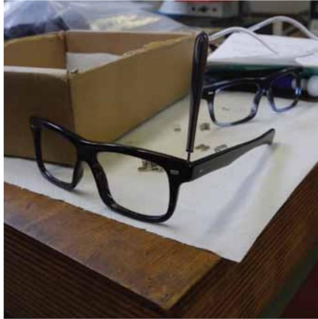
The pantoscopic angle is tested and checked, this is an important part of the quality control.
