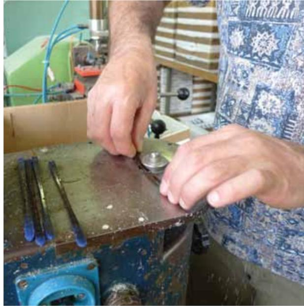
The edges of the templates are shaved down to remove harsh edges.
