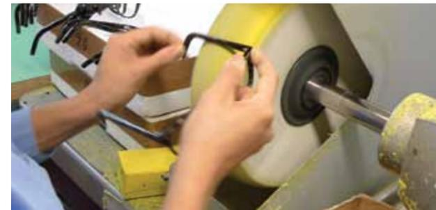
The frames are washed ultrasonically and once dried the frames are taken to the polishing room where a four step process of polishing begins.
