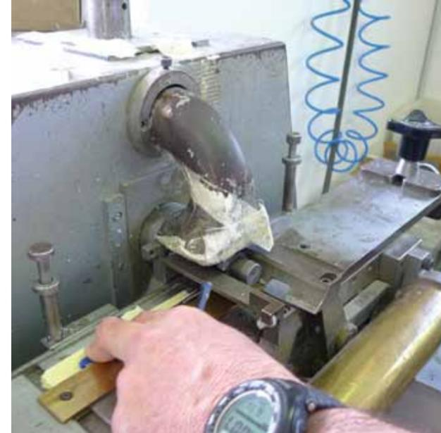
Once the temple has been shot it has its thickness reduced. As with the frontals we may only have 6mm acetate instead of 4mm which would be too thick and heavy to wear.
