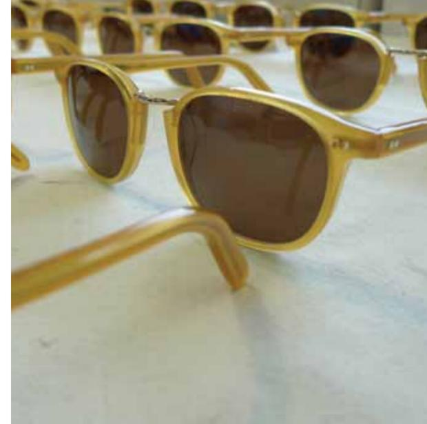
Throughout the final steps there is a visual checking of each frame for scratches, mistakes or faulty components. It is always important that the high Cutler and Gross standards are maintained.
