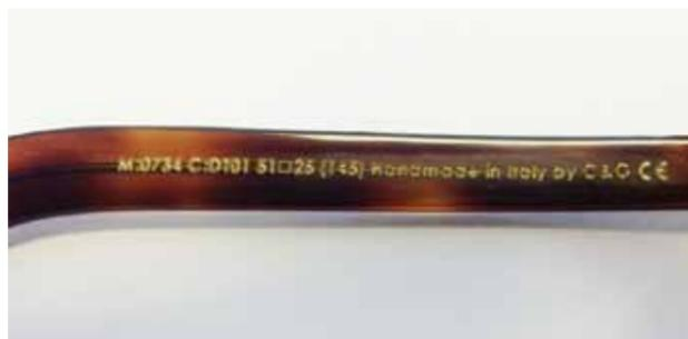
Once these details have been lasered onto the frame the graves are filled with gold ink and carefully polished to highlight the details.
