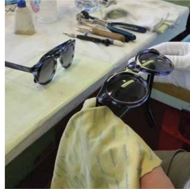
Each pair is carefully and skillfully balanced to ensure they can be displayed and presented properly. Uneven temples can create an uncomfortable fit and will not fit well and appear uneven.
