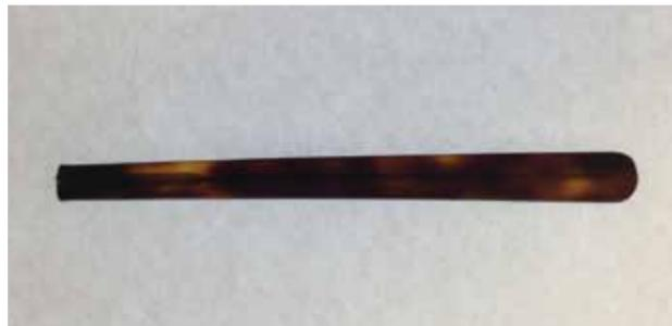
Temples are stamped out of 4mm acetate. A fustella, which is a cutter, is created like a cutter and using heat slices the temples out of the acetate. We currently have over 60 fustellas.
