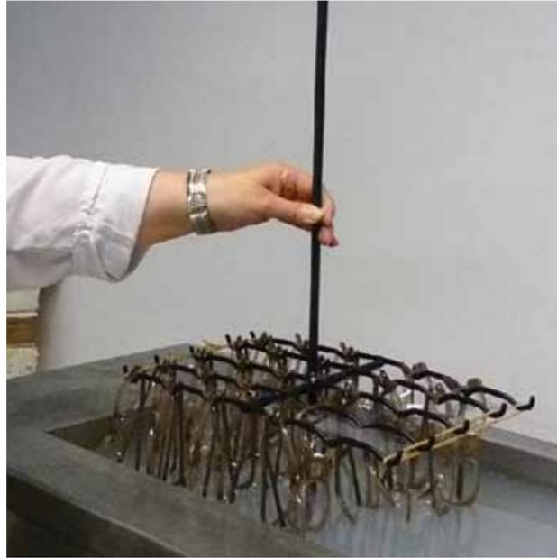
Once the third stage of tumbling is complete the frames are all removed and counted. They are then placed in an ultrasonic bath for three minutes at 30° and then left to air dry.
