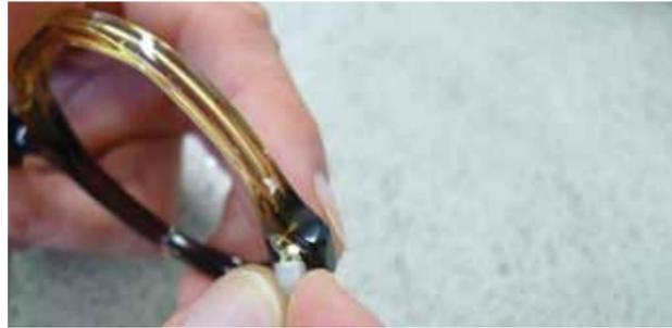
Frontals are next cleaned with a brush drill and an acetone bath. Then, before the tumbling process begins the hinges of each frame are capped with plastic hoods to ensure they are not damaged during the process.
