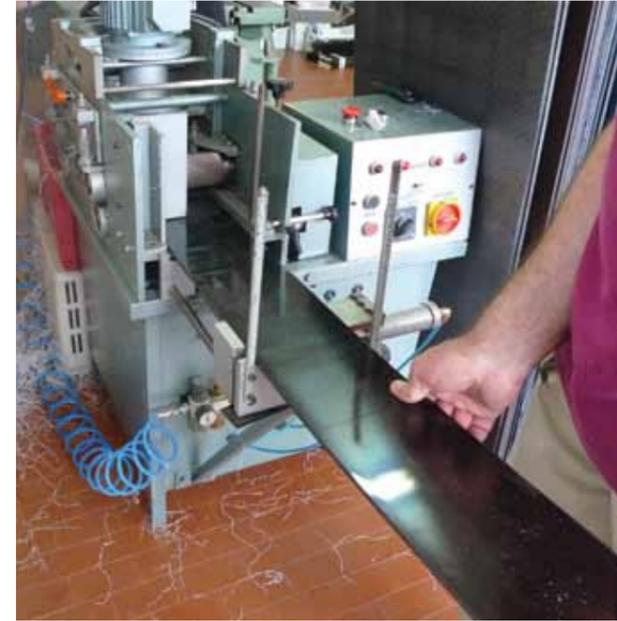
Once cut into strips, all acetates including thicknesses need to be reduced on the thickness plainer as they are not all even when they arrive. Thickness is also reduced when we need 6mm thickness for a frame but only 8mm thickness is available to order. However, since the acetate is ordered in kilograms this extra waste adds extra costs.
