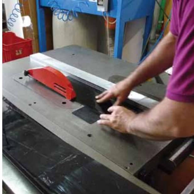
Once received, the strips are cut down to the specific size needed for the frame. Depending on the layout of the print and the width of the strips, the factory endeavours to minimise waste where possible.
