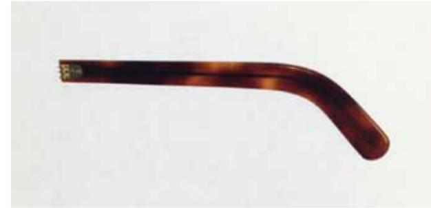
To bend the temple by hand a mould is created which ensures the correct angle is created on each temple. The temples are heated and then bent by hand.
