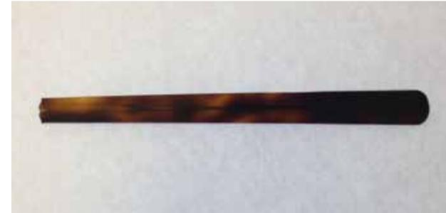
The temple is put into a vice to keep fastened in place for the shooting of the metal core. The central section of the temple is heated and then the metal anima is shot into place.
