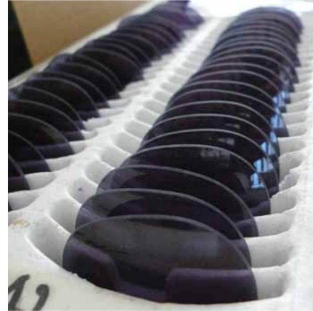
The main companies we currently use to glaze our frames are Zeiss, Dalloz and Intercast. It is very important to select lenses which are compatible with acetate as some materials such as polycarbonate can react with and crack the acetate when placed in one of our frames.
