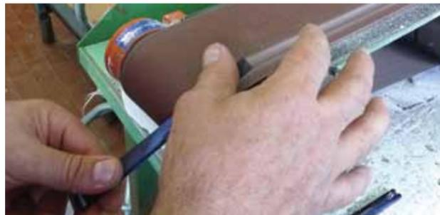
Resin is used to seal the logo within the grave, and then finally this is cleaned up by smoothing the excess resin away with a sanding belt.
