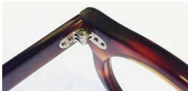
Using an electronic drill the hinges are joined together with specific screws.
